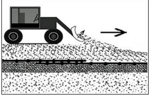
Figure 1: Geogrid overlapping and fill spread direction
